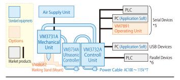
\*5 Spec. of serial (RS-232C) cable is as follows. Vector's VM7873 Cable (5m) meets the specifications.
